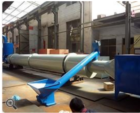
Rotary Drum Type Flash Drier Machine for Moisture of 20-65%
